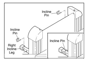
Adjust the left incline leg in the same manner. Make sure that both incline pins are inserted from the direction shown.
